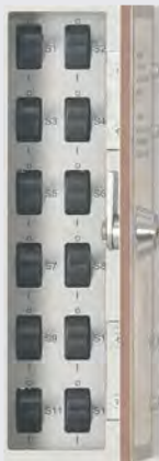
Error Simulator with 12 Error Options via Switches
