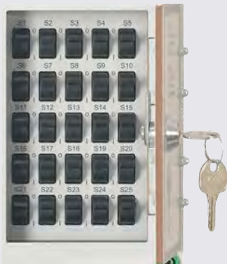
Error Simulator with 25 Error Options via Switches
